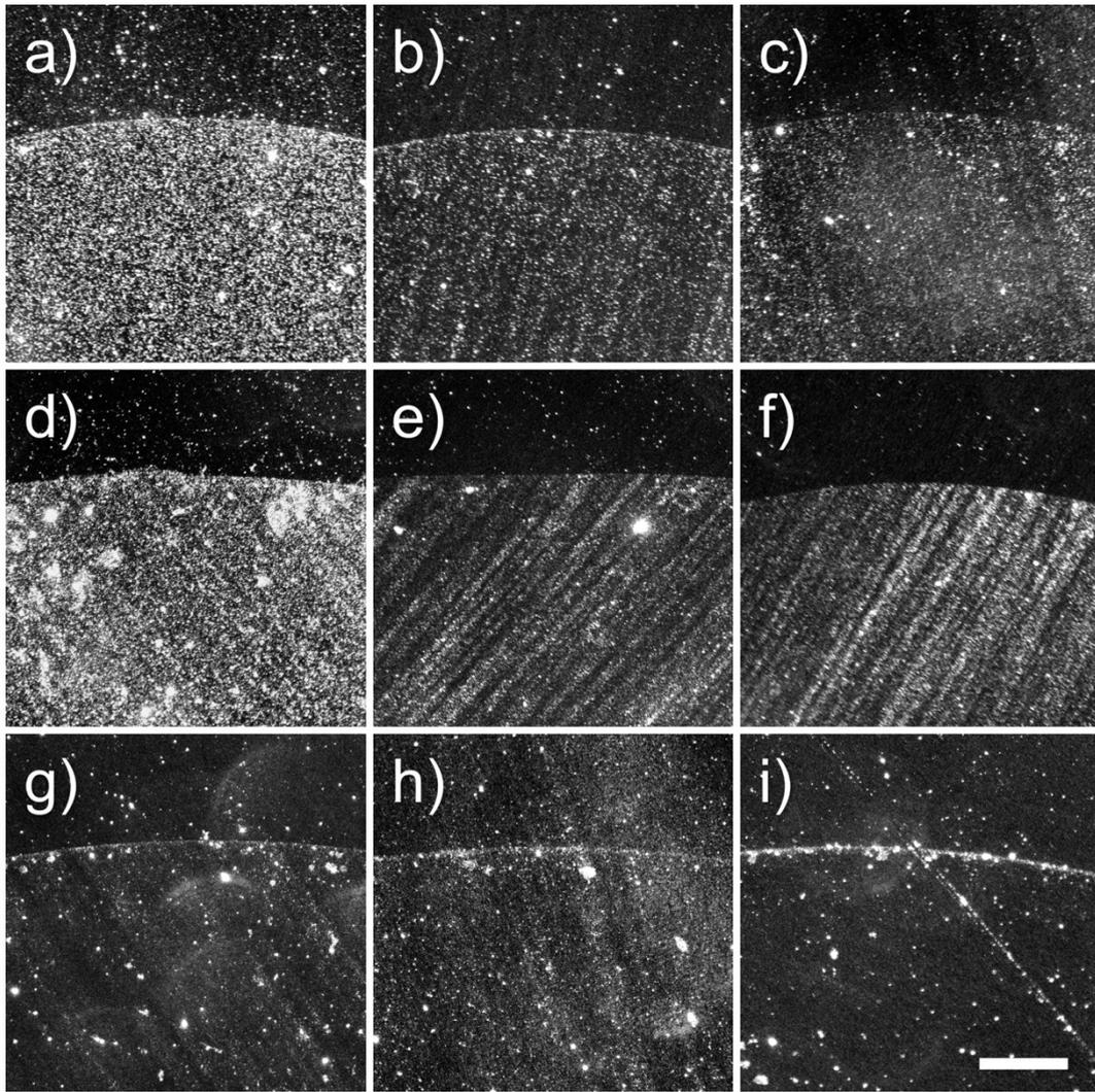
Fig. 3 a-h) NED-VD images of spots edge observed at 20× magnification after incubation with positive samples with corresponding Ct values of 14, 16, 17, 18, 19, 20, 21, 23, respectively; i) NED-VD image of a spot after incubation with negative sample. The scale bar is the same in all images and corresponds to 100 μm.
