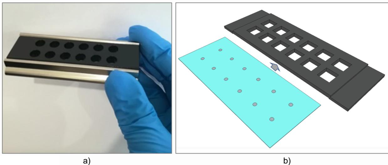
Fig.1. a) Reaction chamber for the coverslip with 12 separated wells. b) Coverslip ready to be inserted in the support for NED-VD reading.
